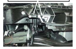
10. Loosely assemble driver's side inner and outer brackets using 2 x M8 x 30 bolts, spring washers, nuts and 4 x flat washers. See photo. Repeat for passenger side.
