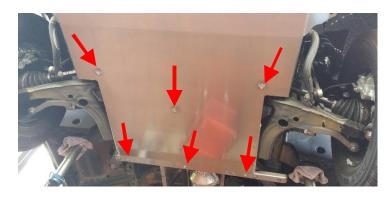
Join the protection plate engine using a gearbox jack on the transverse bar and the assembly carrier and fix onto the transverse bars and the assembly carrier using the 9 M8x35 hex collar screws provided in the delivery. The M8 screws are tightened with 20 Nm.
