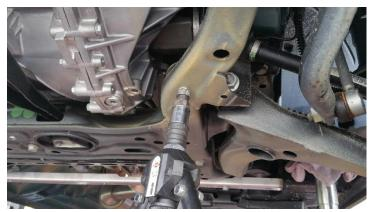
Insert the 3 rivet nuts M8 provided in the delivery in the designated holes of the assembly carrier and rivet.
