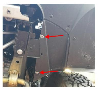
Mount the 4 clamping nuts provided in the delivery on the left and right of the wheel housing liners, as shown in the image.
