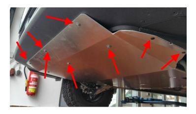
As described in the installation guide 1461 0027, finally tighten both the M10 screws from the transverse bar at the back with 30 Nm.
