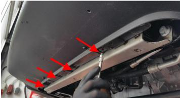
Re-fix the bumper on the crossbar below the cooler using the fixing clips.
