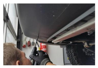
Drill the front 3 marked points on the bumper with a 10 mm drill machine. Drill the rear two markings with 8 mm drill.
