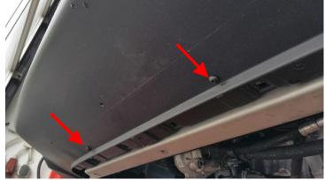
Fix the counterholder to the bumper through both the rear holes using the 2 lens head screws M6x20 provided in the delivery.
