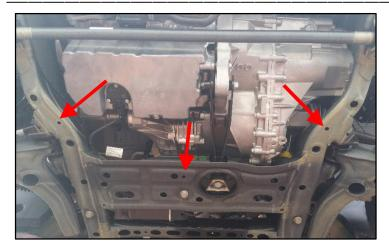
On the image, the 3 fixing points of the protection plate are marked on the assembly carrier: the 3 rivet nuts provided in the delivery are inserted here.
