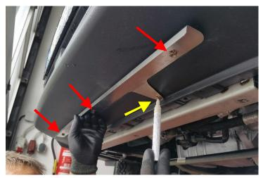
Hold the counterholder provided in the delivery, as shown in the image, on the bumper and align the 3 holes in the counterholder to the markings on the bumper.
