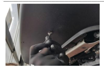
All the 5 drilled holes in the bumper must be deburred.
