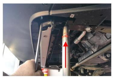
Using a gearbox jack, press the assembly carrier upwards and then tighten the hex collar screws M12x50 as per Volkswagen manufacturer's specifications using 70 Nm and turn 90° further.
