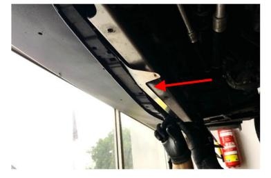
Move the counterholder with the chamfers upwards behind the bumper and align to the earlier drilled holes.
