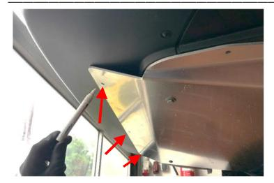
Temporarily fix the protection plate and mark the postion of the front 3 holes on the bumper. Then dismount the protection plate again.
