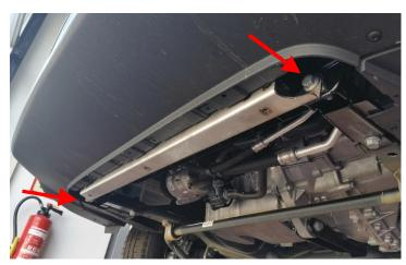
Join the transverse bar provided in the delivery from front at the bottom to the assembly carrier and tighten using the hex collar screws M12x50 provided in the delivery on the left and right.
