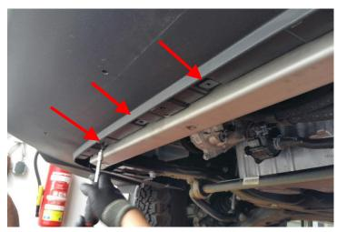
Loosen the fixing clips of the bumper on the crossbar below the cooler.
