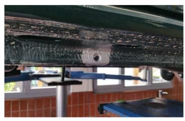
Deburr all the drilled holes and protect against corrosion, as described on page 2.
