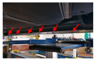
After the anti-corrosion protection is dry, position the rock slider on the rocker using the two gearbox jacks and align. Set the channel section on the inside on the rock slider and screw using
