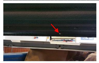
Remove the rock slider profile and the channel section from the rocker. Drill through the marked points on the notch of the rocker using a 4 mm drill from inside to outside and then drill from outside to inside up to 11 mm.
