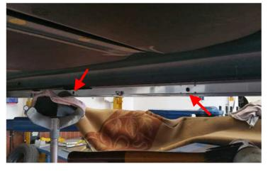
Put the channel section from the inside on the rock slider profile and fix using two M8 counter-sunk screws and nuts.
