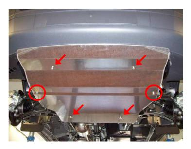
Fix engine protection to the original threaded inserts on the assembly carrier using 6 M8x60 screws.
