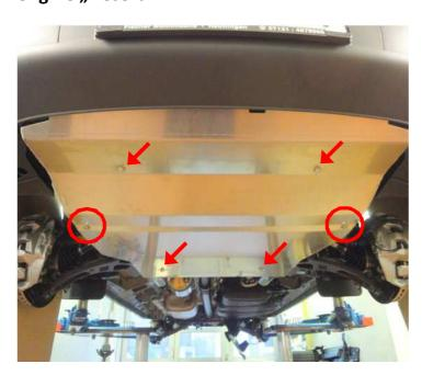
Fix engine protection to the original threaded inserts on the assembly carrier using 6 M8x60 screws.
