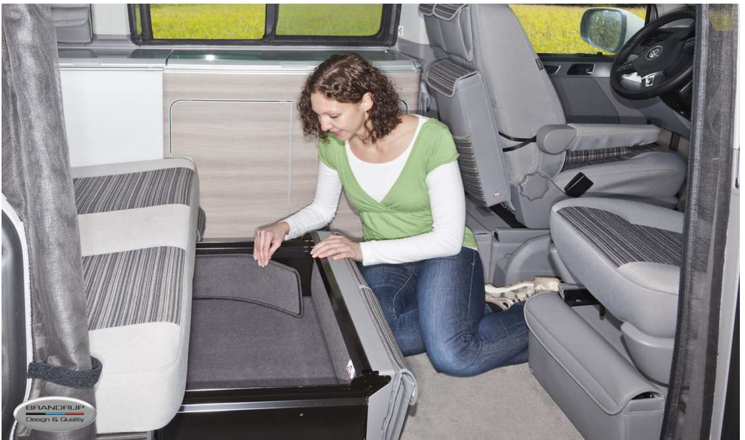
Noise damping mat and set T6.1/T6/T5 California: ideal to reduce noise inside the drawer beneath the bed (2-seater bench): deposited items do no longer "rattle" and are better protected. The awning crank can still be clipped in. The noise damping mat (floor) is simply placed into the drawer. The noise damping set (side parts) is attached with hook-and-loop fastener.
