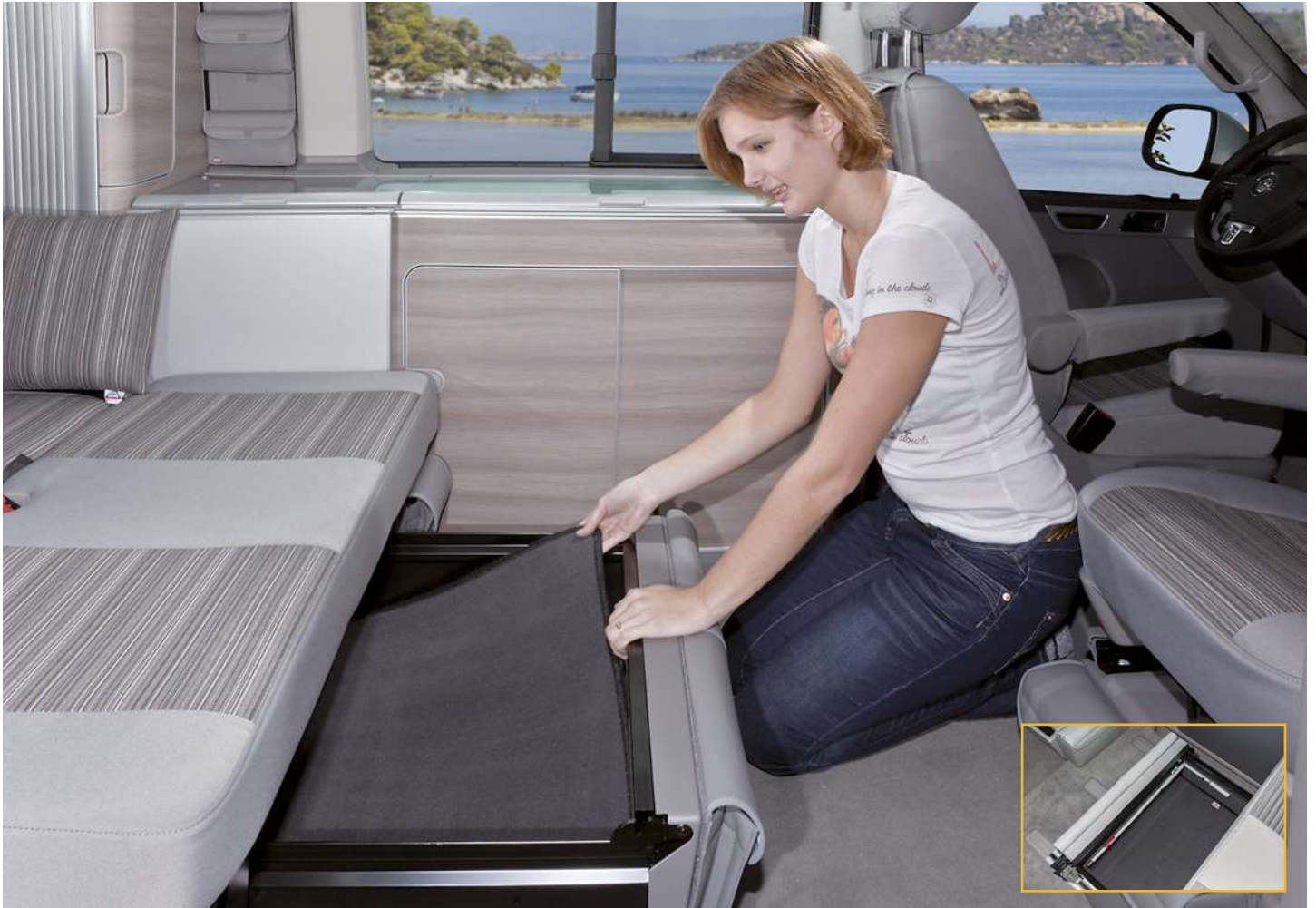
Noise damping mat and set T6.1/T6/T5 California: ideal to reduce noise inside the drawer beneath the bed (2-seater bench): deposited items do no longer "rattle" and are better protected. The awning crank can still be clipped in. The noise damping mat (floor) is simply placed into the drawer. The noise damping set (side parts) is attached with hook-and-loop fastener.
