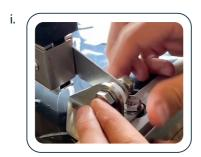
D. Tighten the nut but leave enough space so that the ladder can move freely.
