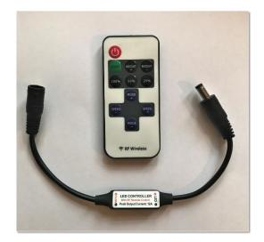
The LED Controller is attached between the short cable from the Light Box and the cable to the power adapter.
