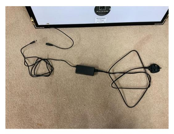
The power adapter is 9.5 x 4.5 x 3cm. It provides a12V, 3A supply to the Light Box, which draws  $\sim$ 30W.
