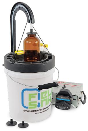
FieldSink being used as a low-flow station. Geopump peristaltic pump, tubing and sample bottles not included.
