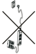
Do not use multiple power strips, which may cause overheating or fire.
