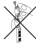
There should be no foreign matter or wire entanglement on the wire.
