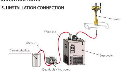
Connect the plug after all connection are compceted
