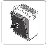
3 Remove the carbon filter from the filter case.
