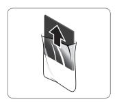
S After removing the packing vinyl of the filter, insert the carbon filter into the filter case.
