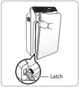
Remove the filters from the unit, they are protected inside a plastic wrap
