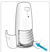
⑤ Replace the back panel by first inserting the latch at the bottom edge into the base of the unit, then rotate the panel upward toward the top of the unit until the panel snaps into the unit.
