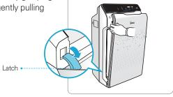
② Remove the filters from the unit, they are protected inside a plastic wrap
