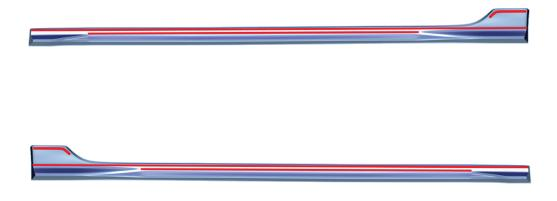
You can now move the side skirts into position. Start with the screw connection at the front wheel arch.
