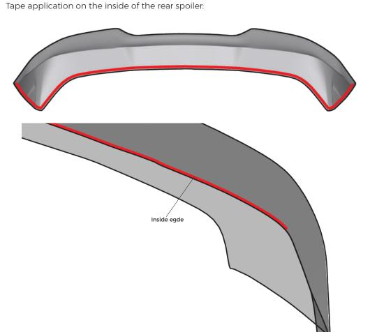
Pull the ends of the tape slightly from 6-8cm. Do not pull the tape off completely to make the installation easier.
