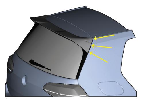
Now press the corners of the spoiler lightly against the car. Once again, make sure that the gaps are even. You can now carefully pull out the protective film of the tape from under the rear spoiler. Press the spoiler firmly against the surface where the tape is placed.
