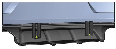
You can now fit the spacer sleeves between the diffuser and the steal holders. Put the long threaded screw through the holes in the middle of the diffuser and the sleeve and screw it into the threaded sleeve.
