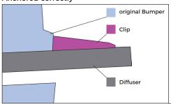
(3) INSTALLATION OF THE DIFFUSER
