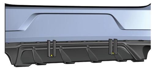
You can attach our diffuser now. Make sure that all tabs are inserted correctly in the original bumper.
