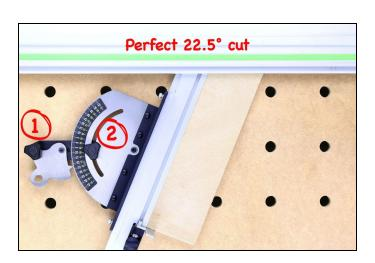
**6**. Precision Mighty Miter can be placed on the right side of the Guide rail (splinter guard side). Calibration will need to be done against the splinterguard edge. This setup with a fence of your choosing is very handy in doing angled cuts on some short pieces as miniature picture frames etc.
