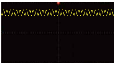
DC+AC Vdc=50V, sine ripple Vac=5V, frequency 150Hz
