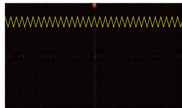
DC+AC Vdc=50V, triangle ripple Vac=5V, frequency 150Hz
