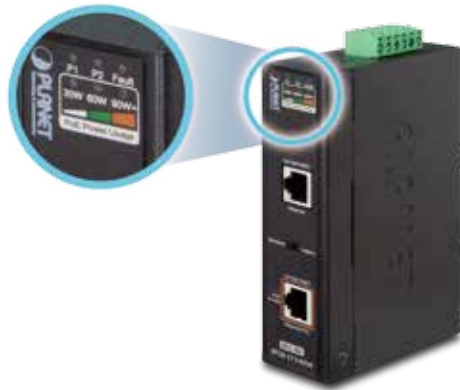
Power Input and PoE Power Usage Display
