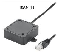
The EA9111 Spot Fluid Leak Sensor is designed to reliably monitor a remote location for the presence of water or any other conductive liquid. The sensor can be extended (up to 30m) using a standardRJ-45 coupling.
