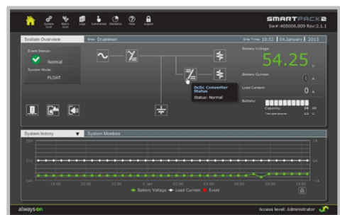
STATUS OF DC/DC CONVERTERS IN SMARTPACK2 WEB
