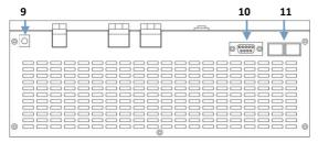
9.AUX DC OUTPUT: Output terminal providing DC power source to the optional
