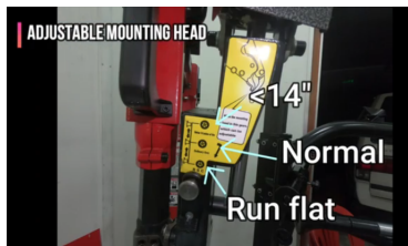
ADJUSTABLE MOUNTING HEAD
