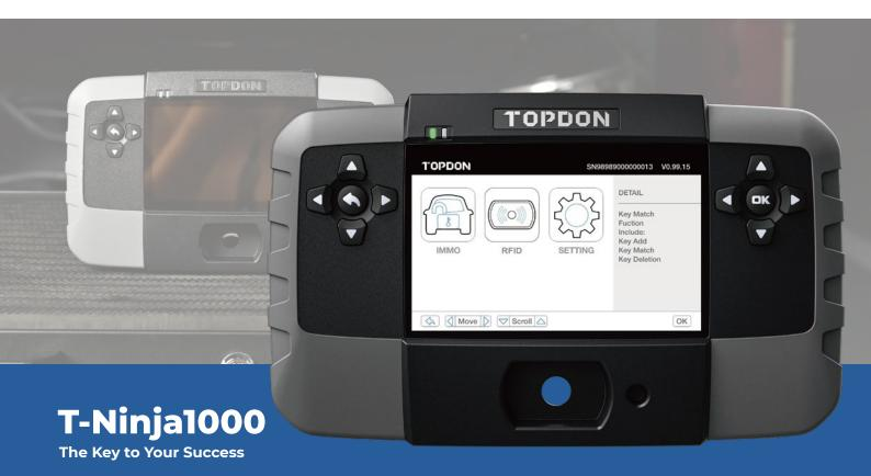
The T-Ninja1000 is an OBDII key programming tool for the automotive immobilizer system. Its integrated RFID Induction Slot diminishes human error and picks up data instantly, making your workflow more efficient. With a real-time guided operation and built-in tips and hints, this product will minimize your downtime and speed up your work. This cost-effective device maximizes its value with so many practical functions.
