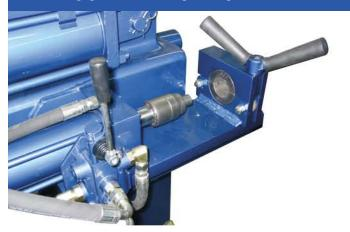
The unique gripper clamp feature two-piece collars with double-tapered walls to eliminate pipe slippage during expansion and reduction operations. The greater the force exerted on the tube, the tighter the grip is. This unit is designed for use with solid dies to perform many different forming operations, slip fits, domes, flares, ball joints, flanges and reductions.
