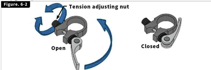
**Please Note**: If necessary, tighten the clamp by twisting the clamp handle clockwise while in the un-clamped position. Then, fold the handle in toward the seat post. This should require a fair amount of force to ensure the seat post is held tight. If necessary, the clamp can be further tightened with a 5 mm Allen wrench while in the clamped position.
