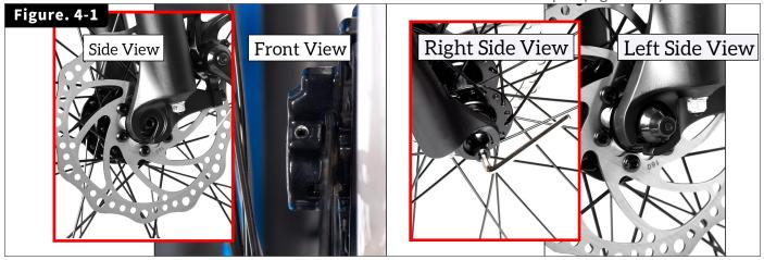
2. Insert the quick release axle (Note: The small spring heads face the center and one on each side of the wheel). Use the Allen Wrench to tighten the nut of the quick release(Figure. 4-2).
