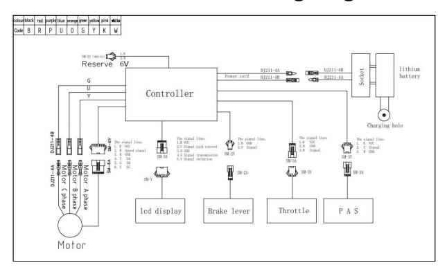
This wiring diagram is only for reference, if any question you have, please contact customer service for any repair.
