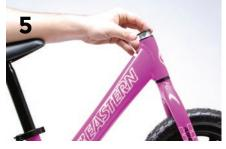
5. Once the fork is completely inserted into the frame place the top bearing spacer on the fork tube.
