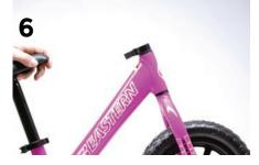
6. Place quick release on the fork tube making sure the quick release tightens towards the front of the bicycle.
