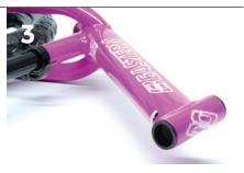
3. Ensure that both nylon bearings are inserted fully into the frame. If they are not completely inserted tap them lightly until the shoulders are flush with frame.
