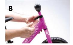
8. Adjust to the desired height making sure the split in the fork and the adjustment area on the quick release are aligned.
