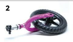
2. Notice the quick release and two bearing spacers on the fork tube.
