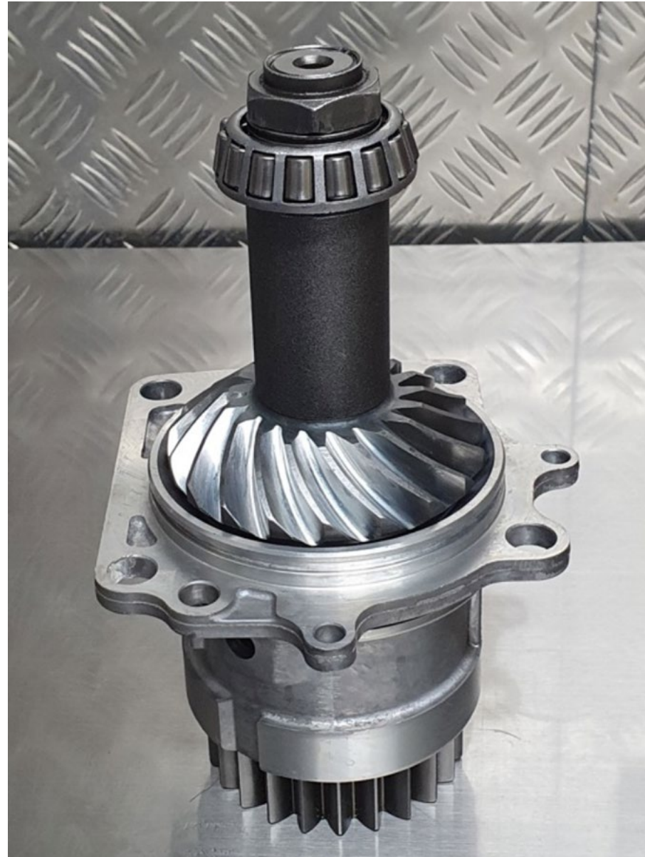
FIG 6 Drive wheel Input OEM housing assembly ready for assembly
