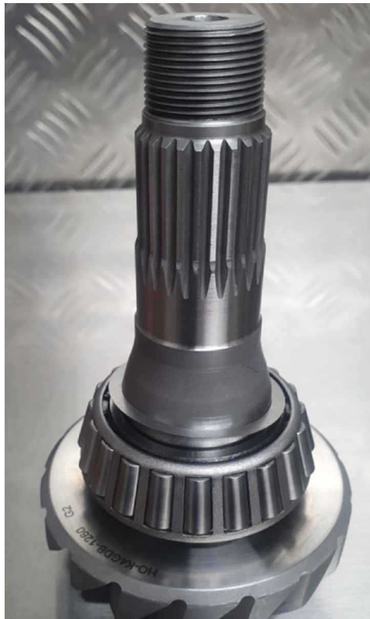
FIG 11 Installing the correct measured shim for 2nm preload
