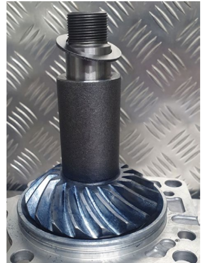
FIG 12 The supplied billet spacer installed
