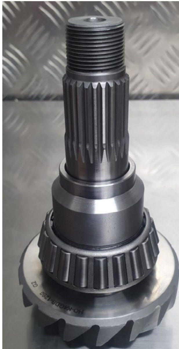
FIG 12 The supplied billet spacer installed
