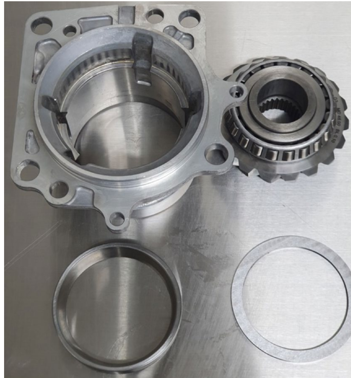
FIG 5 Drive wheel Input OEM housing & hypoid gear and heavy duty bearing and cup with 2.14mm steel shim
