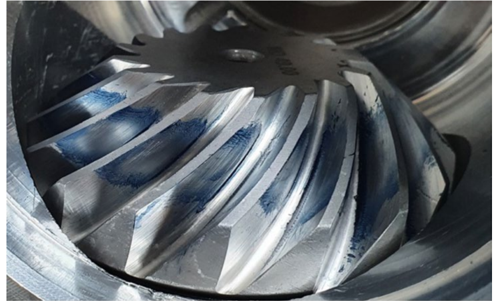
FIG 9 This indicates a good central tooth face contact patch and correct shim thickness for optimal performance. Need to try and not use, toe contact, flank contact, heel contact & face contact, unless you are directly describing the outcome based on the images from page 11
