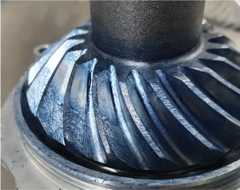
FIG 8 Engineers blue applied to highlight the installed contact patch. Optimizing this contact is key to longevity
