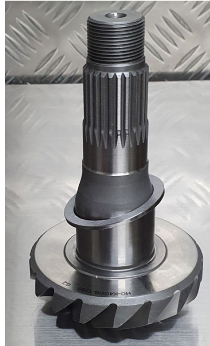
FIG 2 Hypoid gear driven wheel & 35mm spacer
