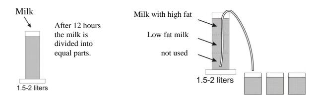
Milk with high and low fat is used for auto calibration of milk analyzer.
