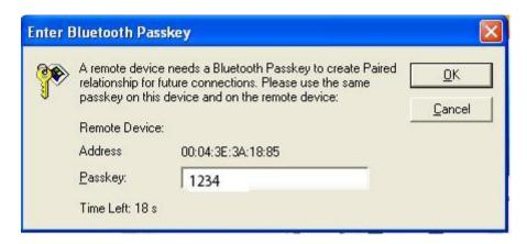
After setting up the connection, on the computer the following message will be shown for a moment (on the picture below). The transfer of data will be through "Serial Port (COM54)" in the case shown on the picture.
