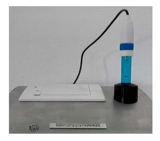
Connect the electrode to the pH connector on the rear panel of the analyzer. Now when you start measuring milk, the device will automatically measure pH of the milk sample.
