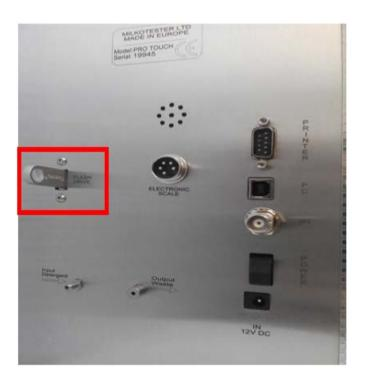
Lactomat BiSonic has internal memory for 500 measurements and has the option to send all saved results to flash drive.
