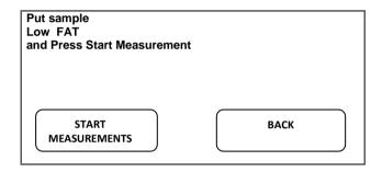
The sample of milk with low *Fat* must be measured 5 consecutive times. Put the first cup with the sample and press ENTER. After measurement the following text appears on the display:
