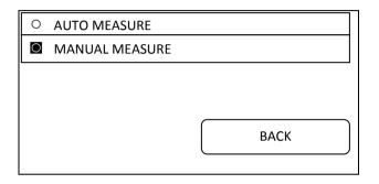
Under the manual mode, the milk sample is put under the pH probe, then you press the pH button and the measurement will last without interruption (until the pH button is pressed again). In order to measure pH the device must be in a working condition.
