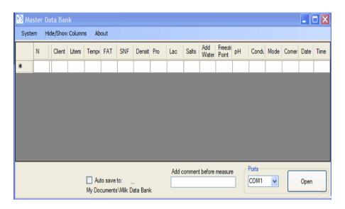
In the down right corner of the window you can see the COM PORT that is connected milk analyzer. Choosing button OPEN, both devices connect each other and every measurement made from the analyzer will be ordered in the table.
