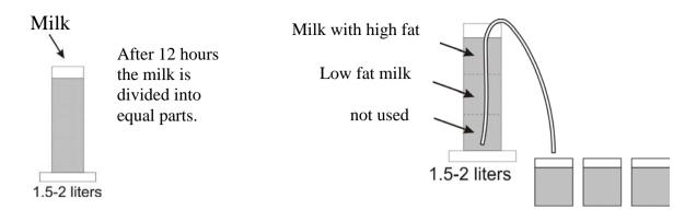
Milk with high and low fat is used for auto calibration of milk analyzer.
