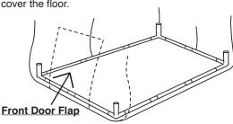
Step 3 - Assemble sides and insert into bottom frame with the bottom of
