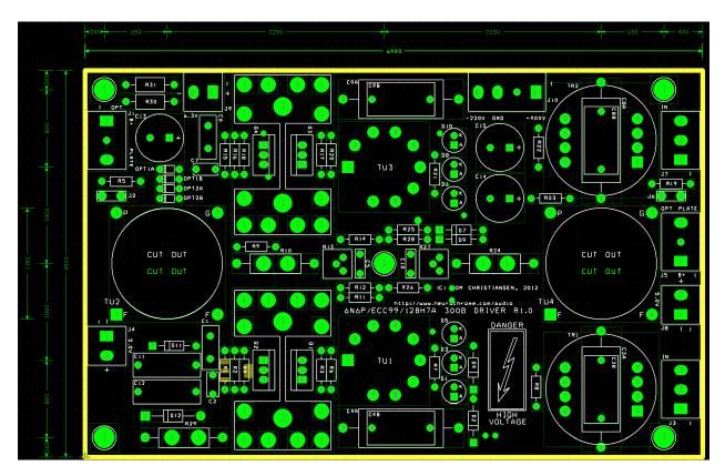
The board is intended for mounting below the top deck of the amplifier chassis. Using 12 mm (or 0.5 ") standoffs allows sufficient clearance for the 9-pin tube sockets. The cutouts allow for the pins of the 300B sockets, mounted to the top plate, to poke through.
