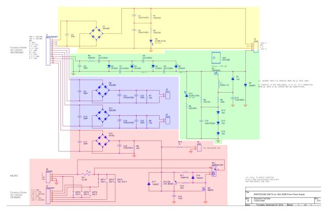
The power supply is comprised of four parts: B+ supply (yellow), bias supply (green), filament supplies (blue), and a soft-start circuit with options for selecting the appropriate mains voltage (red).
