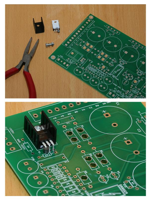
16. Diode bridges: D1, D8, D11. Please observe the polarity on these devices, in particular D1. These devices should ideally be fitted with a small heat sink. A sheet of 1.6 mm (1/16") aluminum  $40 \times 150$  mm (1.5  $\times$  6 inches) is adequate. Another option would be to attach them to the (metal) chassis.
