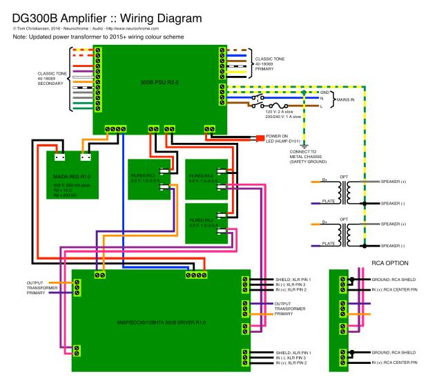
The wiring diagram for the completed DG300B amp using the older model of the Classic Tone 40-18069 power transformer is shown below. These are the connections to use if your Classic Tone 40-18069 power transformer was made in 2014 or earlier.
