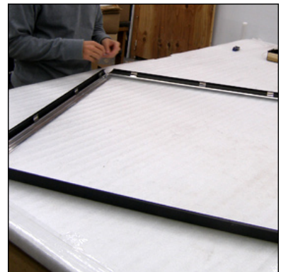
Step 6: Repeat until all Four Mitered Corners are Joined. Then Place Backing Board and Overlay into Frame (If Included) and Snap all 4 sides down.
