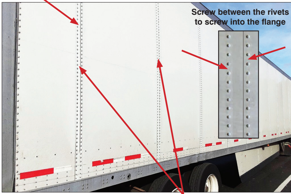
The outer alum or steel "skin" is riveted to "Hat" channels inside trailer.
