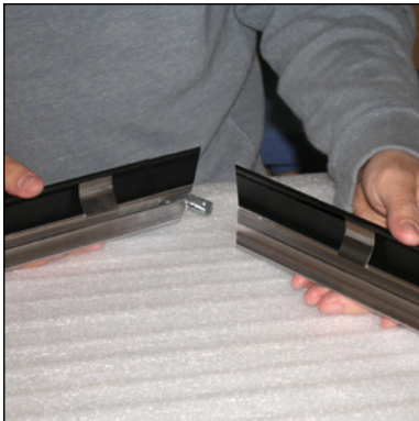
Step 4: Join Mitered Corners. The Hardware Slides Into Slots
