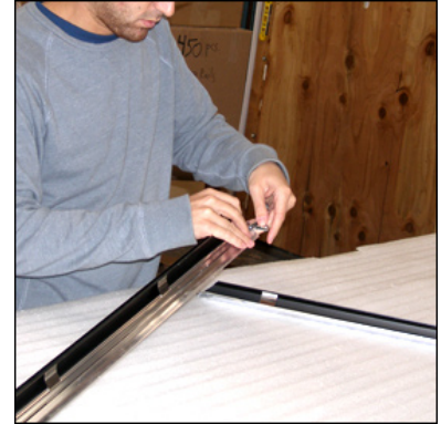
Step 3: Place Hardware Corners into Ends of Mitered Snap Frame Rails
