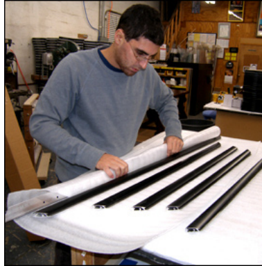
Step 2: Un-Wrap and Snap Open each Frame Rail
