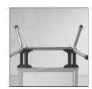
•Connect the top part on to the screws just like shown in the picture.
