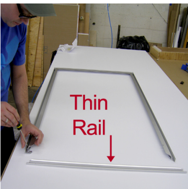
Step 7: When all (3) Large Rails are assembled, tighten the fourth and Final Slot (Thin) Rail. This is the side that the Poster will Slide into.
