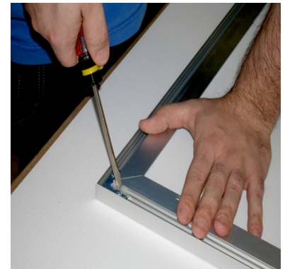
Step 6: Use Philips Screwdriver and Tighten Screws on Hardware. Repeat for all four corners.
