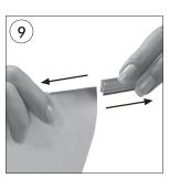
• Slide the plastic clips out in direction of the arrows.
