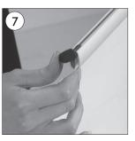
• Slide the plastic clips&poster into aluminium profiles as shown by arrows.
