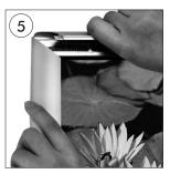
• Close the top profile, side profiles and bottom profile in order. Lock the bootom profile by allen key.
