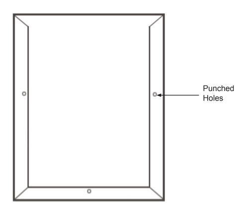
To mount Top / Side Loaders, there are Punched Holes in Back of Metal Frames for Screws. Screws and Wall Anchors are provided.
