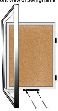
Insert screws through Hanging Bracket and secure into wall anchors
