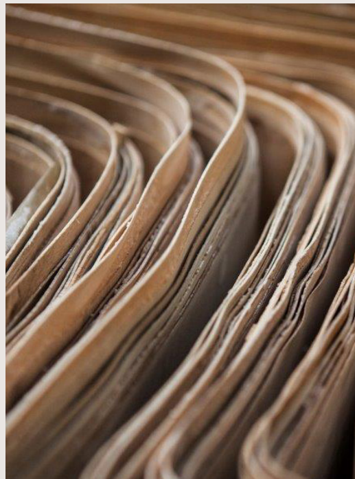
Veneer pieces 3D printed from wood waste
