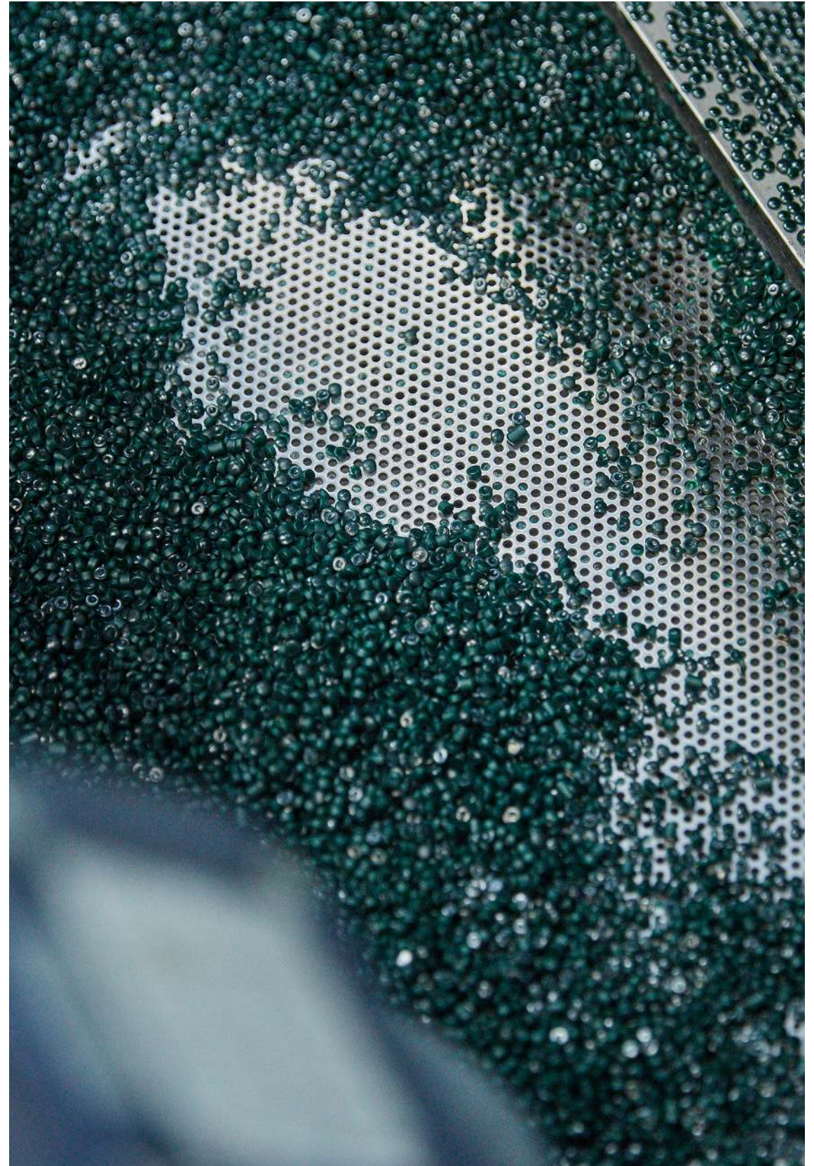
After the fishnets have been washed and cleaned, they are made into small plastic waste pellets called 'Green Plastic'
