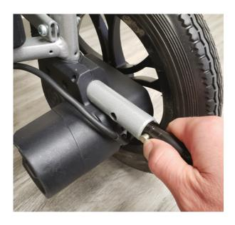
Insert the battery into the left holster position on the back of the power wheelchair. Listen for a \*CLICK\* to ensure it was inserted fully.
