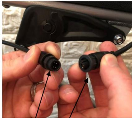
Connect CPU to Controller wire harness
