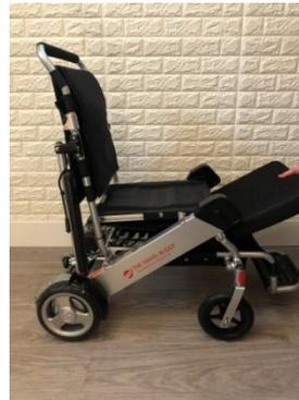
4. Squeeze levers and fold back rest down
