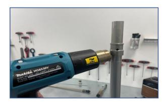
Heat the OEM Cartridge top Hydro stop.
