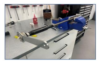
With the FA post securely clamped into the vise use the spring guide and cap, tighten and lock them together on the rod.
