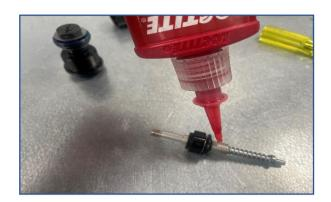
Apply Loctite to the FA Flow Adjuster post.
