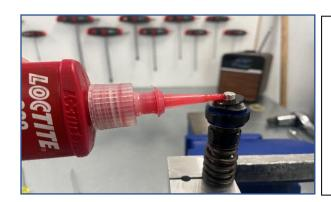
Use Loctite on threads and tension to max 5n or simply nip up gently tight if no torque wrench is available.
