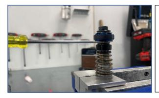
Fit washer and nut gently by hand and check that the lower comp shims float via flicking them down via such tool.
