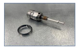
Oem Compression assembly removed and oem piston band
