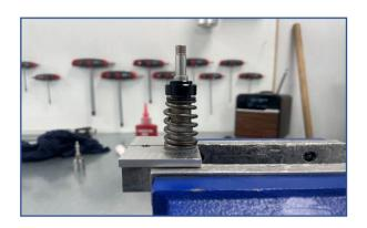
Mount cartridge rod with the FA post installed back into a vice using our 12mm clamping blocks
