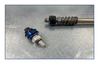
This RHS fork is a lot simpler install. Locate KROOZR Mid-valve post assembly.
