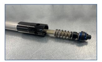
Insert rod back into cartridge making sure the oem piston band does not fall off during assembly.
