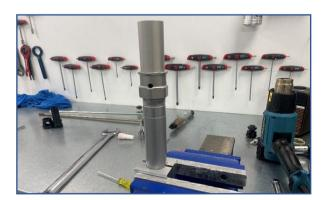
Clamp LHS cartridge in vise as shown. Ensure alloy surfaces of the clamp and cartridge are oil free and dry to allow for a secure clamp.
