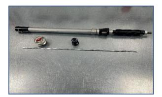
Assemble the rod back into the cartridge and layout ready to install back into the fork outers with our KROOZR compression base valve.
