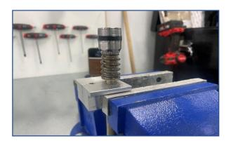
Using our 12mm Shaft clamp, mount the LHS cartridge rod into a vise. We recommend a clean dry rod for best clamping.
