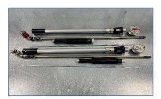
Strip fork down and lay out cartridge parts.
