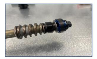
Complete fitted FA post onto LHS cartridge rod.
