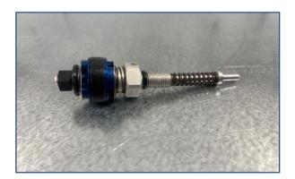
Insert the oem rebound adjuster needle and spring into our Mid-valve post assembly.
