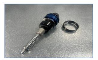
Install Oem piston band to the FA flow adjuster assembly.
