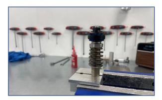
Mount in the clamps in a vise. Tighten using the 17mm flats via spanner.
