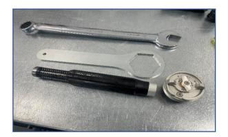
For tightening our post onto the rod using our clamping block you can simply use a 24mm spanner, the OEM spring guide and OEM cap, without sourcing special tools.
