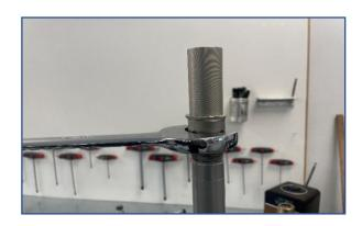
Once quite hot this will loosen the oem Loctite and allow an easy undo using a 32mm spanner.
