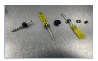
Undo the top nut from our FA post assembly and remove all parts taking care to not mix up any part / install order. We simply slip all shims in correct order onto a small screwdriver or zip tie for ease of reassembly.
