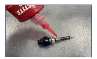
Use Loctite and wind onto the cartridge rod.
