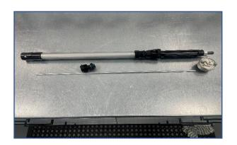
Fit spring seat parts, rebound adjuster rod and wind back on the oem spring guide. This side is ready to install to fork along with our already setup Compression base valve.
