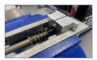
Ensuring the spring and adjuster pin are still inserted to the FA adjuster post wind into the cartridge rod.
