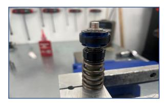
Reassemble all parts back onto the post. See specification for exact order if unsure or have mixed up part order.
