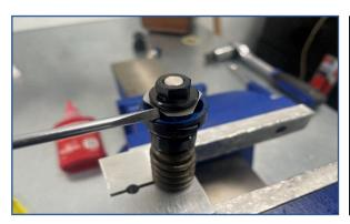
Align all rebound delta shims directly over the piston ports on the rebound face.
