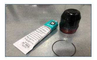
Lube up the inside of the new canister with shock oil or such assembly lube.
