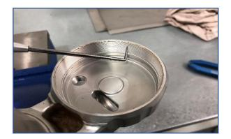
Remove all oem thread lock compound from the shock body.
