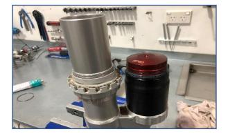
Place Greased bladder assembly into the canister and install circlip. Use a small 4mm bolt or such and pull bladder back up firm against the circlip.
