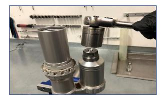
Use Special tool and socket to undo after heating thoroughly.
