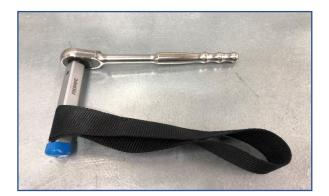
Use Filter strap or any similar strap to tighten the krooztune canister on firm
