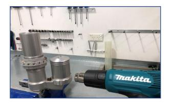
Disassemble the Xplor shock and turn upside down in a vise or such with soft jaws
