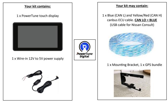
Step 1: Wire-in the power and ground for the power supply. <u>DO NOT POWER THE DASH FROM A CAR STEREO USB</u> <u>OR COMPUTER USB PORT.</u> The dash requires at least 2.5AMPS to power on safely, under powering may damage both the SD card and CPU. It is recommended to wire to the accessories power supply so the screen does not power cycle when the ignition switches between ON and START as you fire up the engine. Unnecessary power cycling is not healthy for the SD card.
