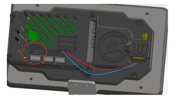
GPS: IF PURCHASED, REMOVE THE SMALL SQUARE HOLDER ON THE RIGHT HAND SIDE OF THE BACK OF THE CASE AND INSERT THE GPS MODULE, IT WILL ONLY FIT ONE WAY. SECURE SCREW, REFER TO THE NUMBERS ON THE GPS HOLDER AND THEN CORRESPONDING NUMBERS ON THE CASE:\_\_\_\_\_\_\_ MATCH the numbers when pinning the GPS wiring to each connector: **Pin 1 to 1 - 2 to 2 - 3 to 3 - 4 to 4**
